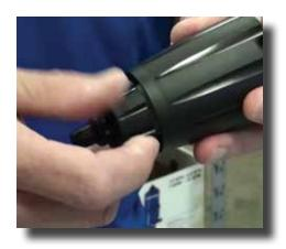
**Step 15:** Next, take the check valve nut and thread it back onto the stem.
