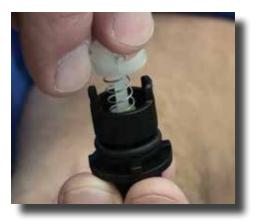
**Step 12:** Replace the retainer (PDI739) by aligning it and turning it a ½ turn clockwise to lock.
