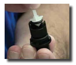
**Step 10:** To reassemble, put the cone (PDI729) back into the check valve.
