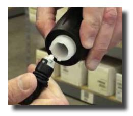
**Step 7:** Pull the check valve straight out. It may be a bit snug, but it will slide out.
