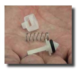
**Step 9:** Once you have the parts out, make sure they are not damaged, gummy, sticky, or missing. If the parts are dirty, you can clean and re-install. But if they are damaged or missing it's time to replace. Remember to keep these parts clean and in good shape so your check valve will do its job.
