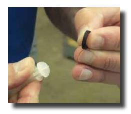
**Step 4:** Set the Medicator down and inspect the plunger seal (J009) for nicks, grooves, or wear.
