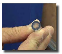
**Step 20:** One last thing . . . take a look at the top of the suction tube. If it looks like it flares out, cut an inch or so off and replace. Or, if the suction tube is cracked, has holes, is rigid, or looks really old, replace.
