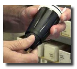
**Step 6:** Now unscrew and remove the check valve nut.
