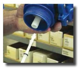
**Step 3:** Next grasp the plunger, twist it ¼ turn counter clockwise. Pull straight out to remove.
