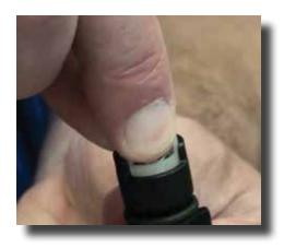
**Step 13:** Before reinstalling the check valve, pull on the top to make sure it stays together.
