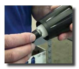
**Step 14:** Reinstall the check valve into the stem.
