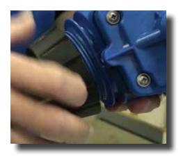
Step 19: Hand tighten the stem nut.
