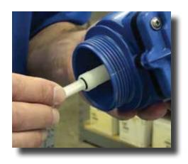
**Step 16:** Insert the plunger into the housing, press it in as far as it will go and twist ½ turn clockwise to lock.
