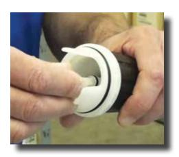
**Step 5:** You can also test by taking the stem and inserting the plunger and then pulling it out. It should make a pop sound. If not or if you see damage, it is definitely time to replace the plunger seal (J009).
