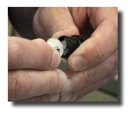
**Step 8:** Grasp the white retainer (PDI739) and twist it ¼ turn counter clockwise to release the check valve parts. Remove the spring and the cone. Inspect the o-ring (JDI105) and replace if worn or scored.
