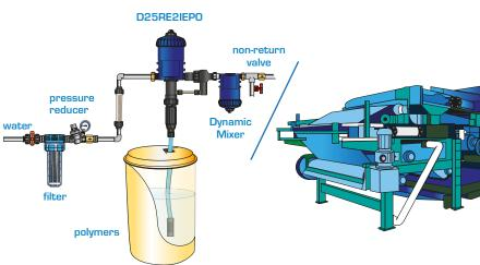
Eloa chose Dosatron as a way to simplify polymer mixing while simultaneously improving the quality of sludge dewatering.
