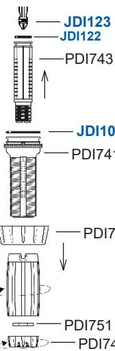
**!** To remove o-ring easily without tools, squeeze it on either side to raise the seal, then slide it over the groove
