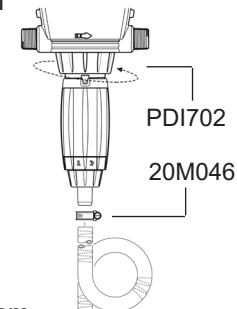
**!** To ensure hose is air-tight, you may choose to carefully cut the top of hose before reinserting.
