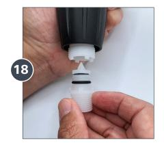
Install the new Check Valve Assembly (Part #: PJDI215) into the stem.
