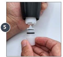
Grasp the white threaded barb and pull the Check Valve assembly straight out.
