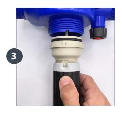
Pull the injection stem straight **down** from the body of the injector.
