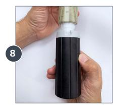
Unscrew and remove the adjusting nut. Set aside.
