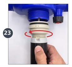
If the scale you prefer is not facing out, just loosen the stem nut and remove.
