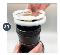
Slide the lock ring and Lower Flange up and off the black piston shell.
