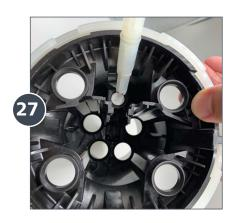
Insert the push rod assembly inside the smaller hole with the top curved portion facing outward (following the curve of the piston).
