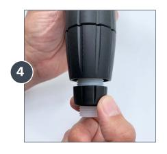
Unscrew and remove the check valve nut.
