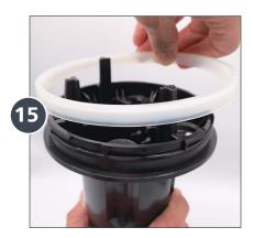
Pick up the NEW **Upper Flange** (**PDI1093**) and slide it onto the piston shell with the **V** shape opening facing downward, and flat edge facing up. Push down until it sits on the ledge of the black piston shell.
