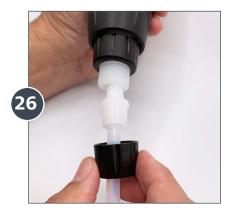
Slide the hose and ferrule onto the barb at the bottom of the Dosatron unit, then tighten the hose nut.
