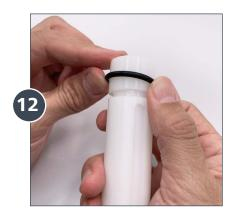
Before placing the insert back into the injection stem, remove and replace the **Injection Stem O-Ring (Part #: JDI120)**.
