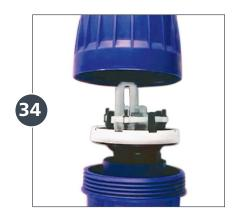
Insert the piston back into the Dosatron injector and screw the bell housing back on.
