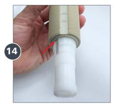
Align the groove in the white stem with the tooth inside the lower portion of the injection sleeve. Slide the stem down as far as possible.
