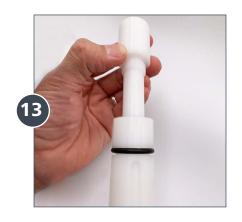
Screw the upper insert back into the top of the injection stem.
