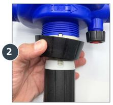
Unscrew the injection stem nut, slide it down and set aside.
