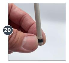
Set the stem aside and pick up the blue body. Remove and replace the **Plunger Seal** (**Part #: JDI200**), by pinching it and rolling out of the plunger or using a small flat blade screwdriver.
