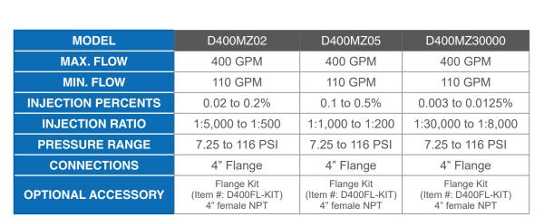
Unit includes: Built-in bypass, externally adjustable injection rate. MAXIMUM TEMPERATURE 104°F
