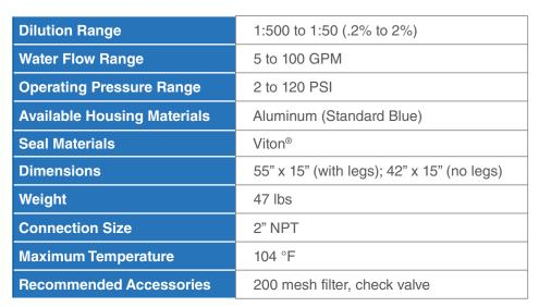
Unit includes: Set of legs, manual bypass, 6 ft clear suction tube, strainer, vacuum breaker and operating manual. MAXIMUM TEMPERATURE: 104°F
