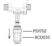
5. Unscrew the locking nut (PDI702) from the injection stem assembly (8CD033) and remove the black anti-rotation lock (PDI751) by spreading it apart, then 8CD033 slide it down
