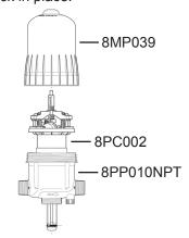
17. Attach the injection stem assembly (8CD033) to the bottom of unit making sure the teeth on the sleeve fit into the grooves of the blue body. Screw the -PDI702 injection stem 8CD033
