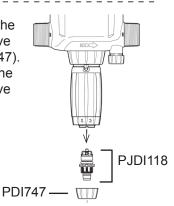
3. Take off the top guide (PDI756) by giving it a 1/4 turn counter clockwise, and discard. Discard the check valve spring (MDI359), check valve cone (PDI752) and check valve cone o-ring (JDI131).
