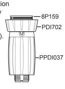
12. Reinstall the "C" clamp (PDI751) by gently sliding it over the threads at the bottom of the white injection stem (PDI753). Screw back the locking nut (PDI733).
