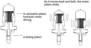
2 clicks = 1 motor \_\_\_\_\_ Once in the up \_\_\_\_\_ Once in the cycle = 1 displacement \_\_\_\_\_\_ position \_\_\_\_\_ down position
