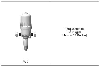
The device can be connected to the water supply line by means of 40 mm interior diameter flexible pipes (drinking water certified, where applicable) fixed with swivel fittings Ø 40 x 49 mm [1 1/2"]. Make sure that the water flows in the same direction as the arrows (water flow direction) on the device.
