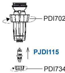
7. Push complete injection stem assembly in position at the bottom of the blue body, making sure desired scale is facing front of injector. Keys at the top of the black sleeve should slide into the slots at the bottom of the body. Slide injection stem nut (PDI702) up the sleeve and screw back on. Insert hose back onto the bottom of the check valve barb. Screw hose nut (PDI735) back on.
