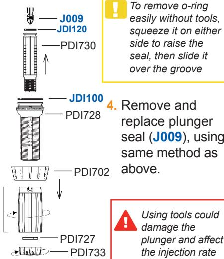
4. Remove and replace plunger seal (**J009**), using same method as above.
