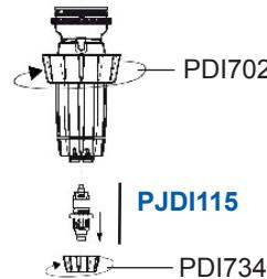
3. Unscrew locking nut (PDI733), remove "C" clamp (PDI727) by slightly spreading the opening and gently sliding it down over the threads. Unscrew adjusting sleeve (PPDI036). Holding the sleeve (PDI728), push up on the threaded part of the injection stem (PDI730) and slide it out of the sleeve from the top. Replace both sleeve and injection stem o-rings (**JDI100** and **JDI120**).
