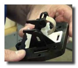
**Step 4:** Remove and replace the slider assembly (PPDI048) that includes the white plastic slider, rocker, and the blade spring.
