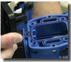
**Step 3:** Remove the black actuator plate. Set the Medicator aside.
