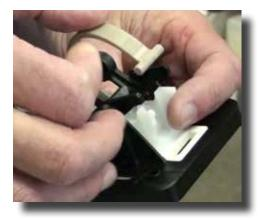
**Step 10:** Hook the blade spring on the rocker and press the axle into the top of the slider.
