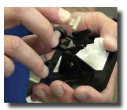
**Step 5:** To begin, press the blade spring and lift up and off of the rocker.
