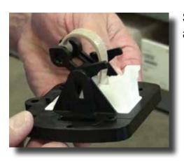
**Step 11:** If you hold the actuator plate assembly with the arrow facing you, the blade spring will curve away.
