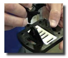
**Step 7:** To remove the rocker, spread the supports and pull it up.
