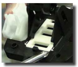
**Step 9:** Align the arrow on the slider with the two arrows on the actuator plate and install the new slider.
