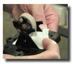
**Step 12:** Test the new assembly by pushing the slider back and forth. It should click each time and not bind.
