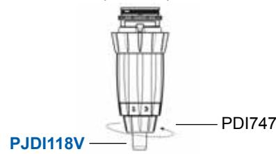
7. Push injection stem assembly in position at the bottom of the blue body, making sure desired scale is facing front of injector. Screw injection stem nut (PDI702). Insert hose onto the bottom of the check valve barb (**PJDI118V**). Attach the clamp (20M046).
