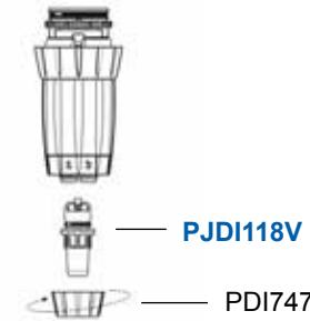
5. Slide the injection stem (PDI743) down into the sleeve (PDI741), making sure the small key located on the bottom inside of the sleeve is properly aligned with the longest groove on the white stem. Holding the black sleeve, pull down on the white stem as far as it will go. Screw adjusting sleeve (PPDI037) back onto the sleeve (PDI741).
