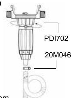
**!** To ensure hose is air-tight, you may choose to carefully cut the top of hose before reinserting.
