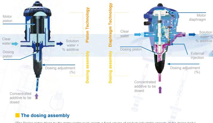
"The Dosing piston driven by the motor continuously injects a fixed volume of product (adjustable capacity of the dosing body). The dosing piston will inject the quantity of product that corresponds to the volume of water passing through the motor. Therefore, the operating principle ensures constant dosing, independently of the variations in flow rate and pressure of the water.
