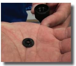
**Step 9:** Replace a new bottom seal (Part #: J003) into the cap, making sure the raised center portion is facing upward.
