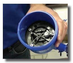
**Step 2:** Grab the metal wishbone and pull the piston straight out.
