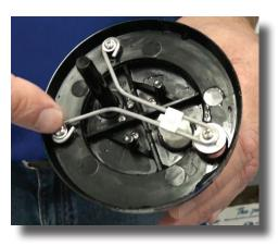
**Step 3:** Set the blue body aside and inspect the wishbone (Part #: MP014) on the top. If anything is broken or missing, replace.
