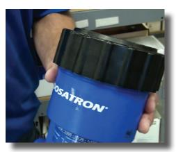
**Step 14:** To finish up, thread the lid on and hand tighten.
