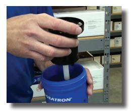
**Step 13:** Carefully insert the piston assembly into the body, pressing it in as far as it will go.
