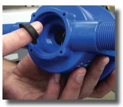
**Step 6:** Remove the top seal that is located between the blue body and the black stem. Please note the top seal sometimes remains in the body. Just remove it.
