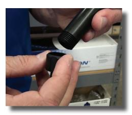
**Step 8:** Remove the bottom seal located in between the black stem and the cap.
