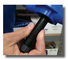
Step 5: Unscrew and remove the stem.
