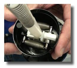
**Step 4:** Inspect the actuator springs (Part #: M009) on the bottom. If anything is broken or missing, replace.
