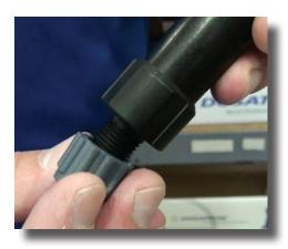
**Step 10:** Now thread the cap onto the bottom of the black stem and reinstall the gray hose nut, hand tight.
