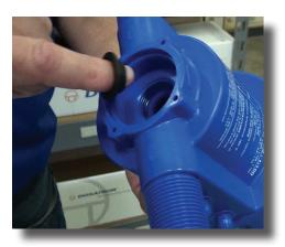
**Step 11:** To replace the top seal, just place it into the body with the raised center portion facing up.
