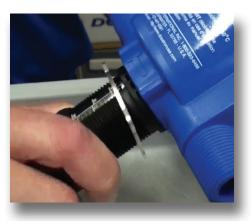
**Step 4:** Pull the injection stem straight out from the body. of the injector. Set the blue body aside.
