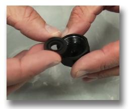
**Step 21:** Place the new check valve seal with the groove facing upward into the new check valve barb.
