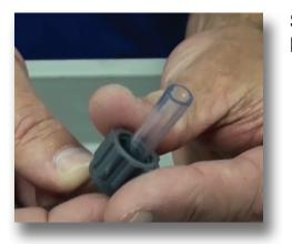
**Step 30:** Now, thread the suction hose nut onto the hose.
