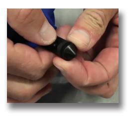
**Step 23:** Pick up the blue unit and remove the plunger seal (Part #: J009) by pinching and rolling it off of the plunger.
