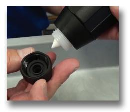
**Step 6:** Remove the check valve seal (Part #: J051).
