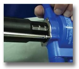
**Step 28:** Place the screws into the body and position the scale on the stem to face outward. Hand tighten the screws in a star pattern.
