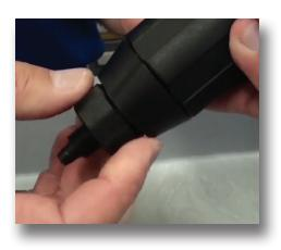
**Step 5:** Unscrew and remove the check valve (Part #: P169) barb.
