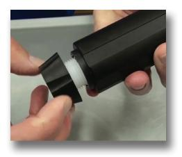
**Step 19:** Slide the anti-lock up and thread on the lock nut hand tight.
