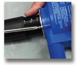
**Step 3:** Unscrew the four screws at the base of the injection stem.
