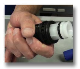
**Step 12:** Push the white injection stem (Part #: PJ121) up and out of the black sleeve and discard.
