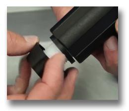
Step 7: Unscrew the lock nut
