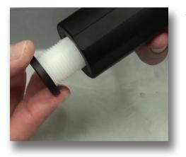
**Step 18:** Install the anti-lock ring by aligning the teeth inside the ring with the grooves in the white stem.
