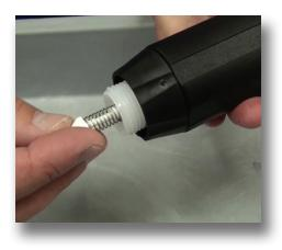
**Step 20:** Now, you can install the new check valve assembly into the stem.
