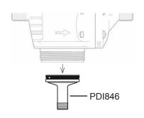
5. Unscrew the check valve nut (PDI734) and remove the check valve assembly (PJDI115), from the injection stem assembly (PPDI045), by pulling it down.
