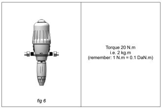
The device can be connected to the water supply line by means of 20 mm interior diameter flexible pipes (drinking water certified, where applicable) fixed with swivel fittings Ø 20 x 27 mm [3/4"]. Make sure that the water flows in the same direction as the arrows (water flow direction) on the device.
