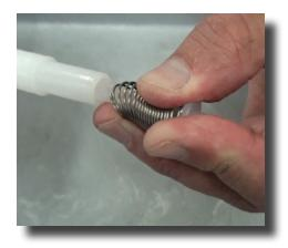
**Step 4:** Install the new slide valve and spring onto the plunger rod. To do this slide the new spring over the top of the slide valve and hold firmly.
