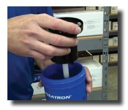
**Step 10:** Pick up the blue body and insert the piston assembly into the body and slide it down as far as it will go.
