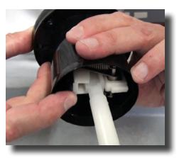
**Step 27:** Test the piston by pressing on the top and bottom of the push rod. It should click both times.
