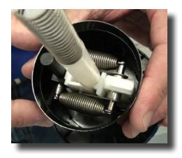
**Step 4:** Inspect the actuator springs (Part #: M009) on the bottom. If you see anything missing, replace.
