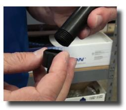
**Step 6:** Unscrew the black cap and remove the bottom seal (Part #: J003) between the black stem and the cap.
