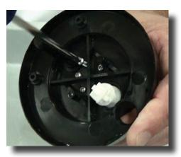
**Step 11:** Remove the four screws in the center of the piston.
