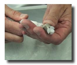
**Step 16:** To remove the slide valve from the plunger rod you will need a large paper clip or awl. Push the spring down and hold firmly.
