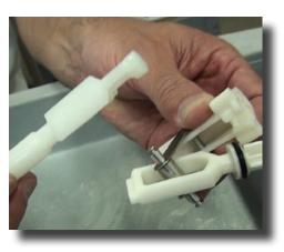
**Step 15:** Remove the plunger rod (Part #: P009) by lifting it up slightly and out. Set aside the actuator (Part #: MP001).
