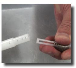
**Step 18:** To reinstall the slide valve onto the new plunger rod slide the spring over the slide valve. Push to the bottom and grasp firmly.
