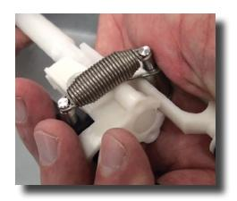
Step 22: Install the actuator springs.
