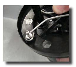
**Step 26:** Reinstall the wishbone spring, then reinstall the washers and screws, hand tight.
