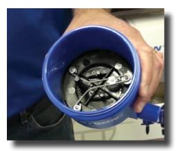
**Step 2:** Grab the metal wishbone and pull the piston straight out. Set the piston aside.
