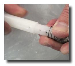
**Step 19:** Insert the plunger and reinstall the pin. The center hole is the 1:128 setting. If you need 1:200, install the pin in the top hole, if you need 1:100, install the pin in the bottom hole. Make sure the pin is flush so the spring doesn't get stuck.
