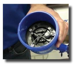
**Step 2:** Grab the metal wishbone and pull the piston straight out. Set the blue body aside.
