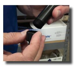
**Step 8:** Insert the bottom seal, raised portion facing up, into the black cap and thread onto the stem, hand tight.
