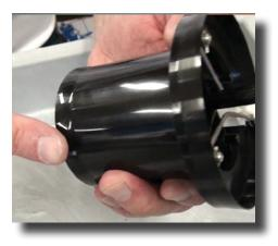
**Step 5:** In order to check the piston shell, remove the piston and check the upper and lower flanges on the piston shell. If they are worn or have scratches the piston shell needs to be replaced.
