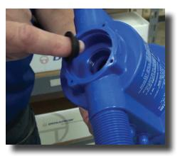
**Step 6:** To reassemble, place the top seal with the raised center portion facing upward inside the body.
