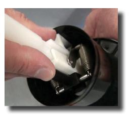
**Step 23:** Align the push rod and inlet valve inside the piston shell and slide the actuator assembly in completely.
