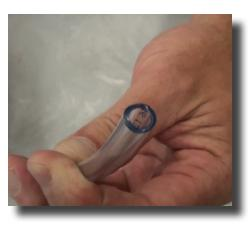
**Step 12:** One last thing. Take a look at the top of the suction tube. If it flares out, cut off an inch or so and reinstall. Or, if the suction tube is cracked, has holes, is rigid, or looks really old, replace.
