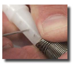
**Step 17:** Now push the metal pin (Part #: M005) out using the paper clip. This allows you to remove the spring from the slide valve.
