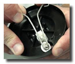
**Step 10:** Spread the wishbone and remove from the inlet valve.
