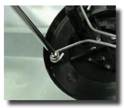
**Step 9:** To change the plunger rod use a # 1 Phillips screw driver and remove the two wishbone screws and washers.
