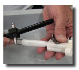
**Step 21:** Install the push rod with the long portion up making sure to insert it with the groove side inward.
