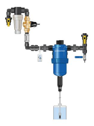
1" polypropylene single union ball valve 1/2" stainless steel ball valve 1" poly 200 mesh tee filter 1" brass pressure regulator w/gauge 1" 20 GPM flow restrictor 1" polypropylene check valve 1" unions schedule 80 PVC 1" x 2" polypropylene fittings 1/2" x 2" polypropylene fittings 1/2" x 1/2" barb fitting 1" to 3/4" reducer bushing 3/4" male to 1/2" female reducer bushing 1" Tee 1" street elbows Roll of Teflon tape Instruction card
