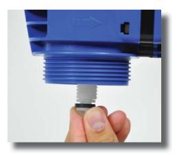
**Step 3:** Pull plunger down and twist 1/4 turn counter clockwise. Pull straight out to remove.
