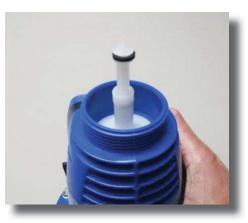
**Step 14:** Push the plunger back into the housing and turn 1/4 turn clockwise to lock. Test the connection to make sure it clicks each time.
