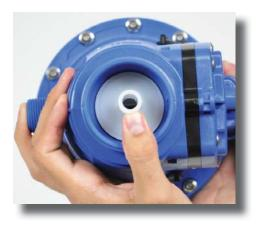
Step 4: Tilt the isolation body and remove.
