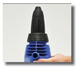
**Step 15:** Reinstall the stem and stem nut. This only has to be hand-tight.
