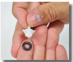
**Step 8:** Remove the spring and the cone. Inspect o-ring (JDI105) and replace if worn or scored.
