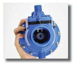
**Step 12:** To reassemble, insert the plunger into the body, twist the plunger a quarter turn clockwise to lock and pull the connector down. Turn the plunger counter clockwise to remove.
