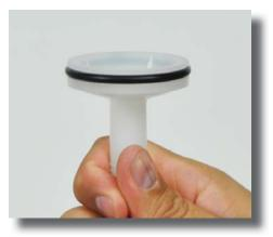
**Step 11:** Inspect the isolation body (PDI846) and o-ring (8J040). Replace if scored or worn.
