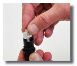
**Step 7:** Grasp white top retainer of check valve (PDI739) and twist 1/4 turn counter clockwise to release.
