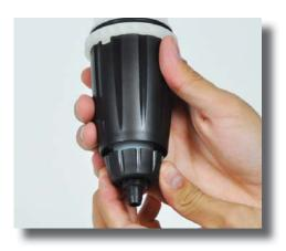
Step 5: Unscrew suction hose nut and check valve nut.
