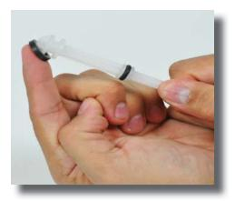
**Step 10:** Remove the plunger seal (J009) and replace. Inspect the o-ring (JDI105) on the plunger and replace if nicked or damaged.
