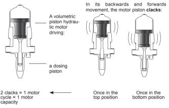
The speed of the motor is proportional to the flow of water passing through the appliance.
