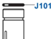
**!** To remove o-ring easily without tools, squeeze it on either side to raise the seal, then slide it over the groove
