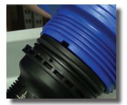
**Step 21:** To finish up align the notches in the lower part of the blue body with the teeth on the top of the injection stem assembly.
