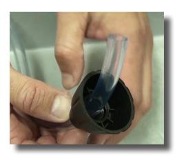
Step 26: Now thread the suction hose nut onto the hose.
