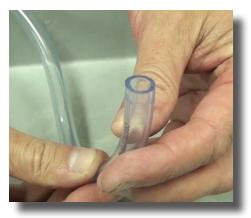
**Step 25:** Before installing the suction hose, inspect it. If it flares out, cut and inch or so off and reinstall or if the suction hose is cracked, ridged, or looks really old just replace it.
