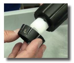
Step 16: Thread on the lock nut and hand tighten.
