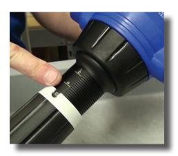
**Step 23:** If the scale you prefer is not facing out just loosen the stem nut and remove. Pull the stem down slightly, rotate and push it back up.
