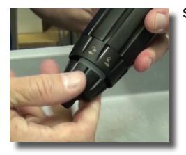
Step 4: Unscrew and remove the check valve nut.
