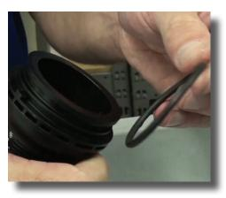
**Step 11:** Remove and replace the sleeve o-ring (Part #: JDI100).
