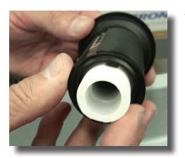
**Step 13:** Insert the white injection stem into the sleeve. Pull it down as far as it will go.
