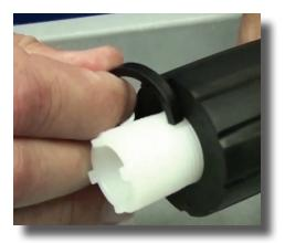
**Step 15:** Reinstall the "C" clamp by sliding it over the threads at the bottom of the white stem. Rotate clamp until it clicks into place.
