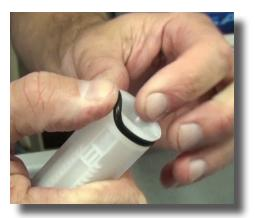
**Step 10:** Remove and replace the injection stem o-ring (Part #: JDI120).
