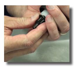
**Step 5:** Grab the barb and pull the check valve assembly straight out.
