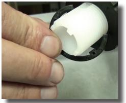
**Step 7:** Remove "C" clamp by spreading the opening and sliding it down over the threads.
