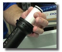
**Step 9:** Push the white injection stem up and out of the black sleeve.
