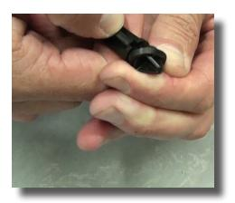
**Step 19:** Set the stem aside and pick up the blue body. Remove the plunger seal by pinching and rolling it off the plunger.
