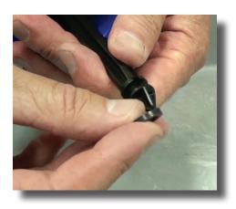
**Step 20:** Install the new plunger seal (Part #: J009) into the groove on the plunger.
