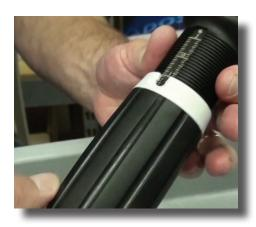
Step 8: Unscrew and remove the adjusting nut.
