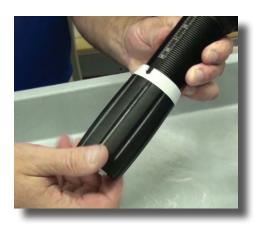
**Step 14:** Thread the adjusting nut back onto the black sleeve.
