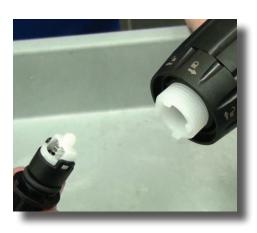
**Step 17:** Insert the new check valve (Part #: PJDI115) into the white stem.
