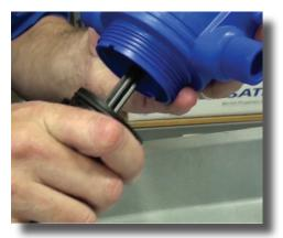
**Step 3:** Pull down on stem to detach from body of unit. Set the nut and body aside.
