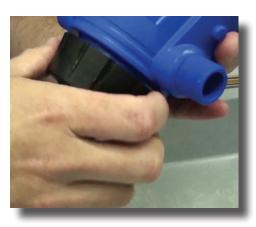
Step 2: Unscrew injection stem nut.
