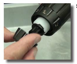
Step 18: Reinstall the check valve nut.
