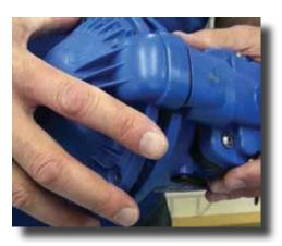
Step 5: Position the lid on top of the housing.
