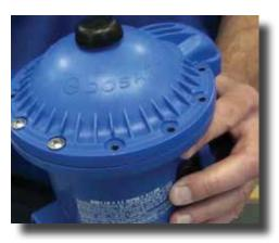
**Step 6:** Install the eleven nuts and bolts, tightening in a star pattern.
