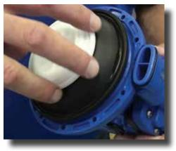
**Step 3:** To remove, unscrew the diaphragm assembly and discard. Install the new part and hand tighten.
