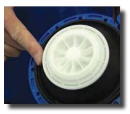
**Step 2:** Inspect the black rubber diaphragm (PJDI127). If it has damage or bleeds off on your fingers, replace it.
