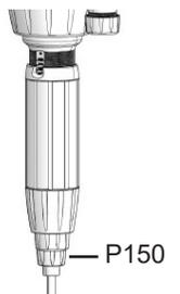
**!** To ensure hose is air-tight, you may choose to carefully cut the top of hose before reinserting.
