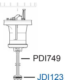
16. Insert the Piston Assembly into the lower housing (PPDI033), then screw the upper bell housing (MPDI186) back in place.
