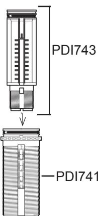
11. Slide the injection stem assembly nut (PDI702) onto the black sleeve (PDI741). Then screw the adjusting sleeve (PPDI037) back onto the black injection sleeve (PDI741).
