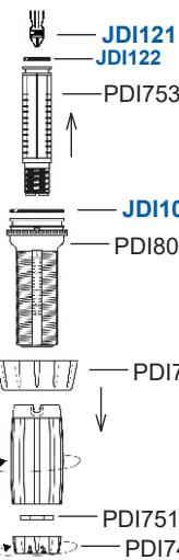
**!** To remove o-ring easily without tools, squeeze it on either side to raise the seal, then slide it over the groove
