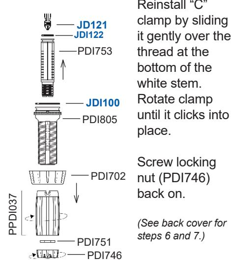
6. Insert new check valve (**PJDI117**) at the bottom of the white stem, making sure that the 4 white keys on the check valve seat next to the 4 black keys on the bottom of the stem. Screw check valve nut (PDI747) back on.
