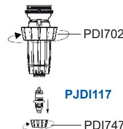
7. Push complete injection stem assembly in position at the bottom of the blue body, making sure desired scale is facing front of injector. Keys at the top of the black sleeve should slide into the slots at the bottom of the body. Slide injection stem nut (PDI702) up the sleeve and screw back on. Insert hose back onto the bottom of the check valve barb (**PJDI117**). Screw hose nut (PDI803) back on.
