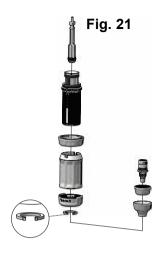
Change the O-ring of the dosing pump body:
