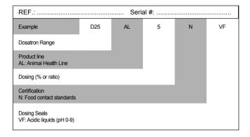
The Animal Health Line dosing pumps with a reference containing the index "N" after the dosing indication are compliant with the regulation:
