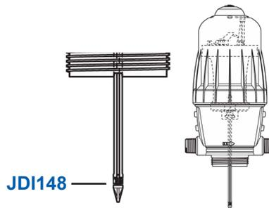
5. Place upper check valve (PJDI063) on check valve barb making sure to insert spring portion down. Insert the check valve (PJDI140) at the bottom of the white stem, the 4 white keys on the check valve should seat next to the 4 keys on the bottom of the stem. Screw check valve nut (PDI734U) back on.
