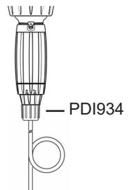
**!** To ensure hose is air-tight, you may choose to carefully cut the top of hose before reinserting.
