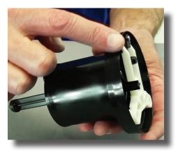
**Step 7:** You can visually inspect the upper and lower flanges on the piston shell. If they are worn or have deep scratches, the piston shell needs to be replaced.
