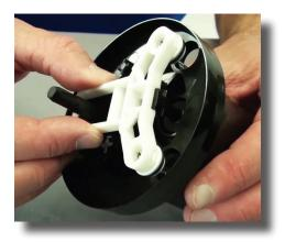
**Step 18:** Reinstall the valve support by sliding it onto the inlet valve.
