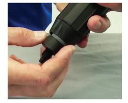
Step 3: Unscrew and remove the check valve barb (Part #: J051).
