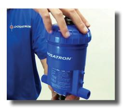
**Step 22:** Hand tighten the lid. The Injector should now be clicking and drawing concentrate.
