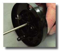
**Step 12:** Next, remove the four screws in the center of the piston shell to release the actuator assembly.
