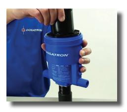
**Step 8:** Also, check the piston shell's fit inside the body. To do this, invert the piston and slide it into the body. It should be a snug fit. If it feels loose, the piston shell (Part #: P421) and the push rod o-ring (Part #: J020) need to be replaced.
