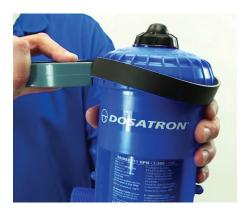
Step 7: Using a strap wrench (Part #: TOOL01), loosen the lid.
