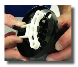
**Step 11:** Then, slide the valve support off the inlet valve and set aside.
