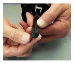
**Step 10:** Take a close look at the plunger seal for nicks, scratches, or wear. If you see damage or don't remember the last time you changed the seal, just replace it now.
