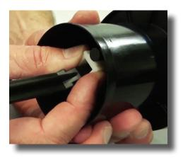
**Step 17:** Press the white plastic portion of the actuator side to side. If there is movement, re-tighten the screws.
