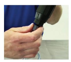
**Step 2:** If there is still no suction, turn the water on. If the unit is clicking, unscrew and remove the suction hose nut.
