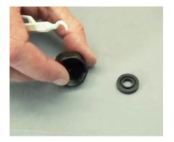
Step 4: Remove the check valve seal.
