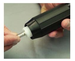
**Step 7:** To reassemble, press the new check valve assembly into the stem as far as it will go.
