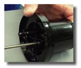
**Step 16:** Now re-install the four screws and hand tighten them in a star pattern.
