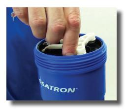
Step 21: Insert the piston back into the blue body.
