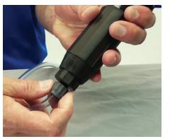
If your Injector is pushing water down into the concentrate container, it's time to investigate the check valve.
