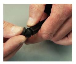
Step 12: Install the new seal (Part #: J009) into the groove.
