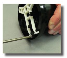
**Step 9:** To replace the piston shell, use a small tip Phillips screwdriver and remove the valve support screws and plastic retainer.
