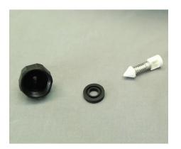
**Step 6:** Inspect the seal (Part #: J051) and the check valve assembly (Part #: MPDI122). If they are dirty, you may be able to soak, brush off, and reinstall. If you see damage or if you don't remember the last time you changed these parts, just replace them now.
