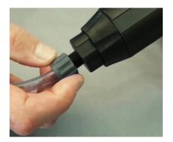
**Step 12:** Hand tighten the nut. This should stop the water from dripping back into the stock tank.
