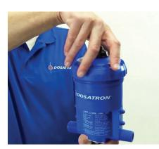
**Step 14:** Replace the lid, hand tight. Your Injector should now be drawing the concentrate. **Step 1:**
