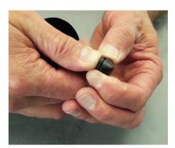
Step 11: To replace the seal, pinch and roll it off of the plunger.
