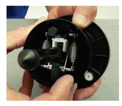
**Step 6:** Then, check the two actuator springs (Part #: M238) on the bottom. If they are broken or missing, just replace them.
