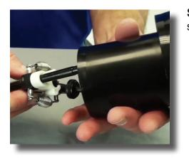
**Step 13:** Pull the actuator assembly out and discard the old piston shell.
