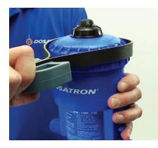
**Step 1:** If the unit isn't clicking, use a strap wrench (Part #: TOOL01) to loosen the lid.
