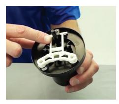
Step 4: Inspect the white valve support on the top.
