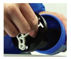
**Step 3:** Grasp the white valve support and pull the piston straight out of the body.
