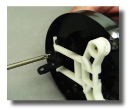
Step 19: Next, position the retainer and hand tighten the screw.
