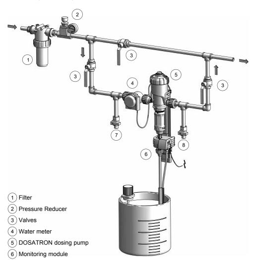
7) Clear water valve: preparing stock solutions & tank rinsing
