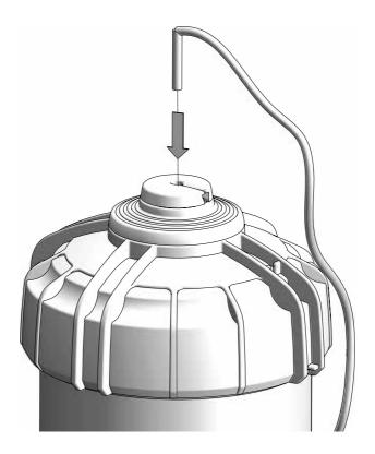
Insert the motor cycle sensor assembly into the centre of the motor lid and insert the cable through the bleed slots and the motor lid.
