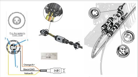
Connect the converter cable directly to a USB port on your computer and follow the installation procedure described in the INSTALLING THE SMARTLINK SOFTWARE section.
