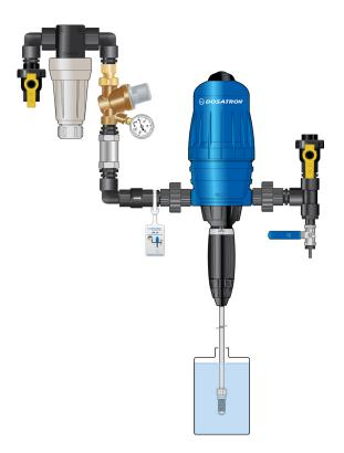
3/4" polypropylene single union ball valve 1/2" stainless steel ball valve 3/4" poly 200 mesh tee filter 3/4" brass pressure regulator w/gauge 3/4" 14 GPM flow restrictor 3/4" polypropylene check valve 3/4" union schedule 80 PVC 3/4" x 2" polypropylene fittings 1/2" x 2" polypropylene fittings 1/2" x 1/2" barb fitting 3/4" male to 1/2" female reducer bushing 3/4" Tee 3/4" street elbows Roll of thread tape Instruction card Zip tie
