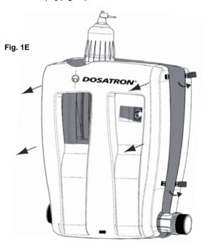
▲ WARNING: If the version being used features an EC probe, open the EC reader and remove the battery protective tab
