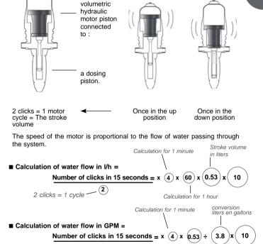
**NOTA**: This method of calculation cannot replace a flow meter. It is given only as an approximate guide.
