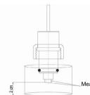
PLEASE NOTE: THE STAINLESS STEEL ELECTRODES MUST NOT TOUCH THE BOTTOM OF THE CONTAINER. THEY MUST BE SUSPENDED 2 CM (1 inch) FROM THE BOTTOM. OTHERWISE, THE MEASUREMENT PROVIDERS WILL BE INACCURATE.
