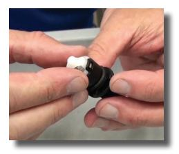
**Step 6:** To change the check valve parts hold the check valve assembly and twist the white top guide (Part #: PDI739) 1/4 turn counter clockwise to remove.
