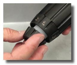
Step 13: Reinstall the check valve nut.
