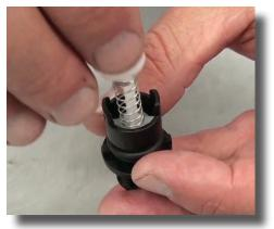
**Step 10:** Slide the new spring over the shaft and position the new top guide over the shaft.
