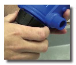
Step 2: Unscrew injection stem nut.
