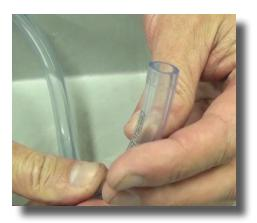
**Step 19:** Inspect the suction hose before installing. If it flares out, cut an inch or so off and reinstall.
