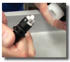
**Step 5:** Grab the barb and pull the check valve assembly straight out. Set the stem aside.
