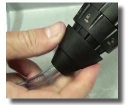
Step 21: Hand tighten the nut.
