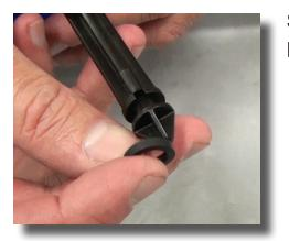
**Step 15:** Install the new seal onto the groove on the plunger.
