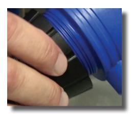
Step 17: Reinstall the injection stem nut, hand tight.
