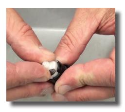
**Step 11:** Align the guide and twist it 1/4 turn clockwise to lock. Give it a tug to make sure everything is in position.
